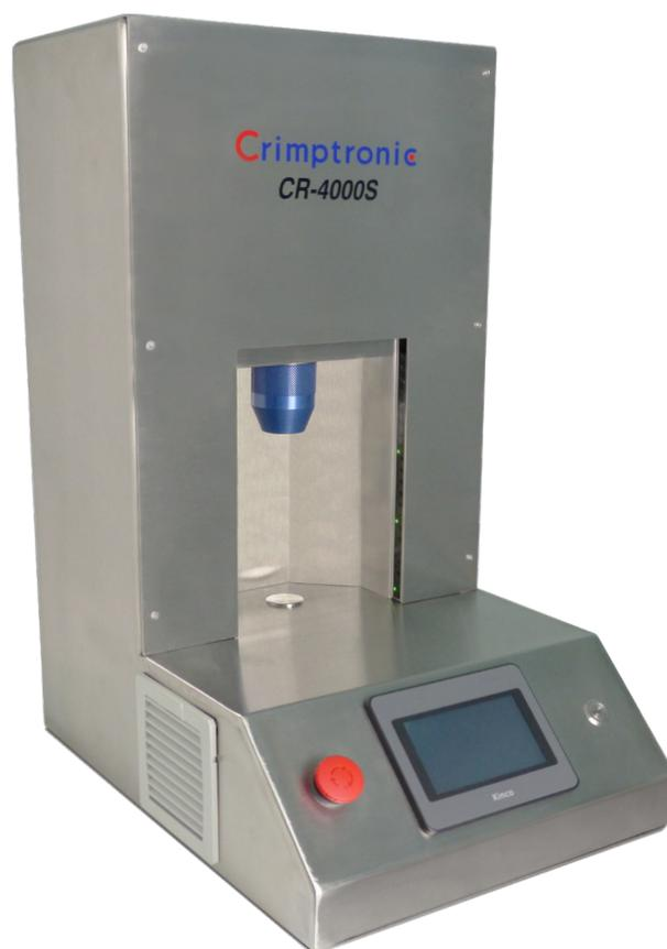
The CR-4000S is versatile, stable, and allows the crimping and decapping force to be adjusted precisely. The interchangeable crimping or decapping heads are easily fitted without tools and are specially suited for crimping and decapping aluminium and steel caps with diameters of 8, 11, 13, and 20 mm, as well as 13, 15, 18, and 20 mm FEA pumps.
